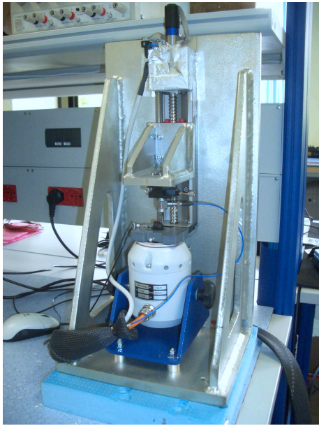
Fig. 11. Experimental setup with dynamic load cell used to measure the response of the sensor. Initial tests have been performed with a shaker moving the fingertip vertically with a sinusoidal profile. The data obtained from one of the receptive fields was compared to the force measured by a PCB 208 C01 dynamic load cell.
