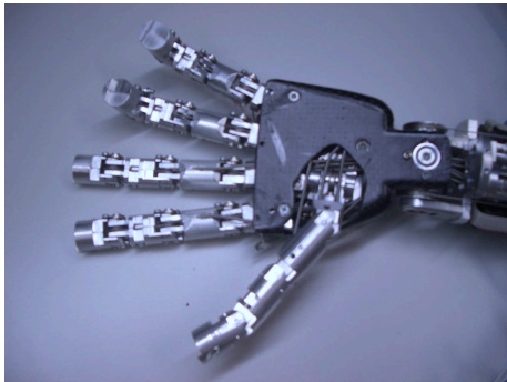
Fig. 2. A hand of the humanoid robot iCub. It has 9 controllable degrees of freedom, not including the wrist, and most of the actuators are located in the forearm.
