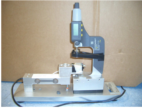
Fig. 8. Test setup with a load cell that can measure static forces. The off-center load cell (3 kg AL series, from Laumas) and the micrometer (TESA Micromaster IP54) are shown.
