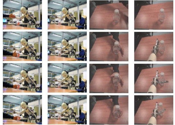
Fig. 11. Grasping an object as performed by an experimenter and the robot. The left two columns show the scene of the action demonstration. The right two columns present the observed action from the viewpoint of the robot.
