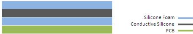
Figure 1. Schematic section of the new architecture proposed for the development of the fingertip of iCub humanoid.
